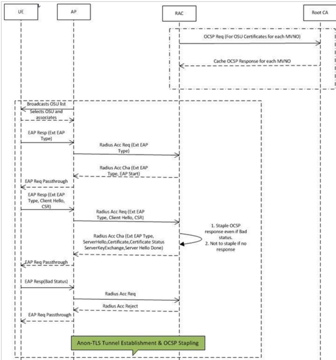
**FIGURE 15** Interaction with OCSP server during EAP-TLS
