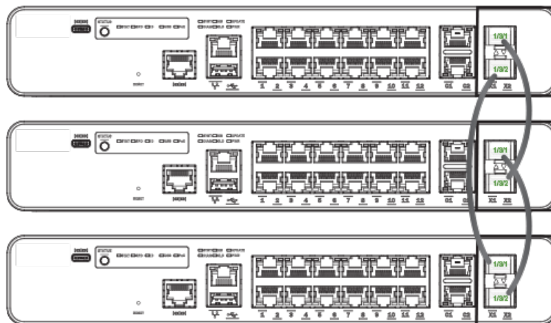
FIGURE 9 ICX 7150-C12P stack ring topology
