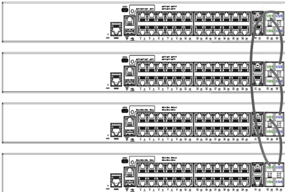
FIGURE 11 ICX 7150 24-port stack ring topology
