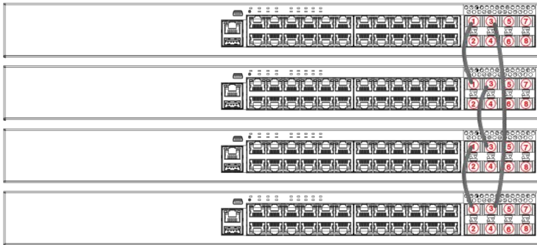
FIGURE 17 ICX 7250-24P ring stack
