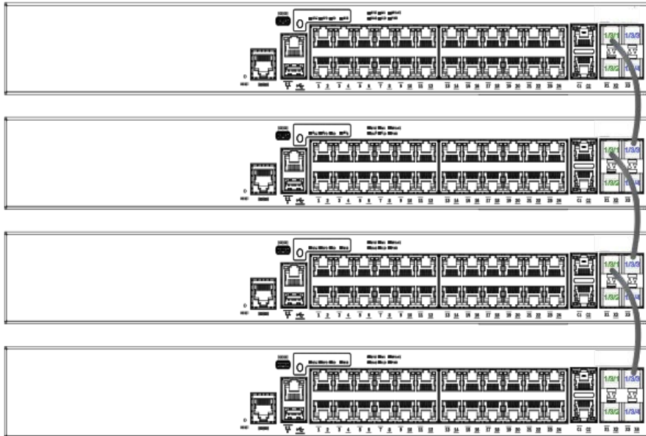
FIGURE 11 ICX 7150 24-port stack ring topology
