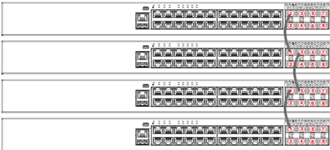
FIGURE 16 ICX 7250-24P linear stack
