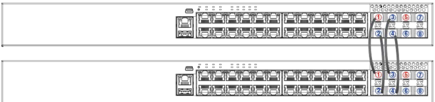
FIGURE 18 ICX 7250-24P two-unit stack with linear-topology trunk
