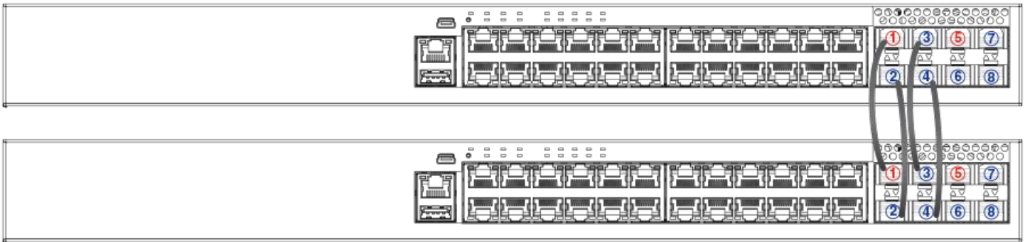
FIGURE 4 ICX 7250-24P two-unit stack with linear-topology trunk as configured in example
