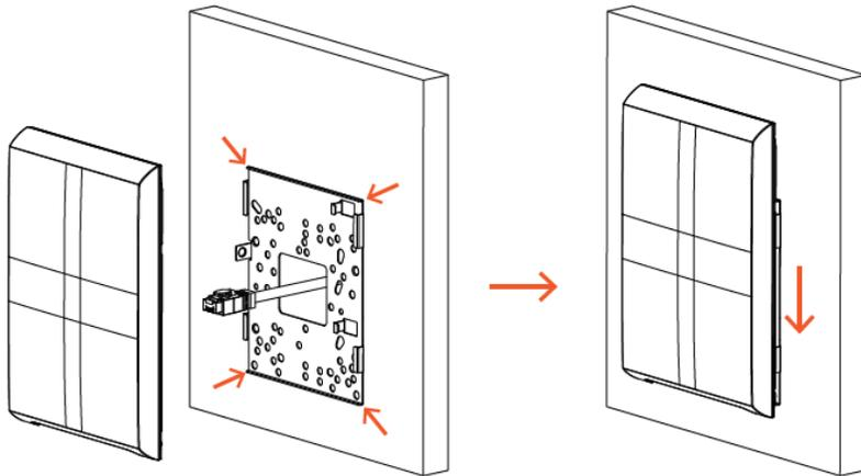
6. Use the bracket screw provided to secure the AP to the bracket.
