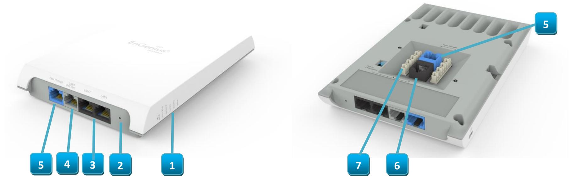
1. LED Indicators: LEDs for Power, Uplink, 5GHz, 2.4GHz, PoE out, Reserve
