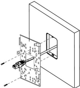
4. Connect the cables to the access point before mounting it to the bracket.
