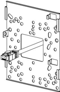
3. Align the mounting bracket with the outlet box and affix the mounting bracket to the outlet box using the original cover screws.
