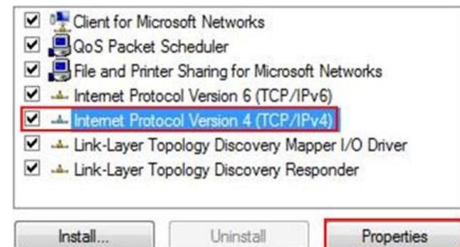
5. Select **Use the following IP address** and enter an IP address that is different from the Access Point and Subnet mask, then click **OK**.
