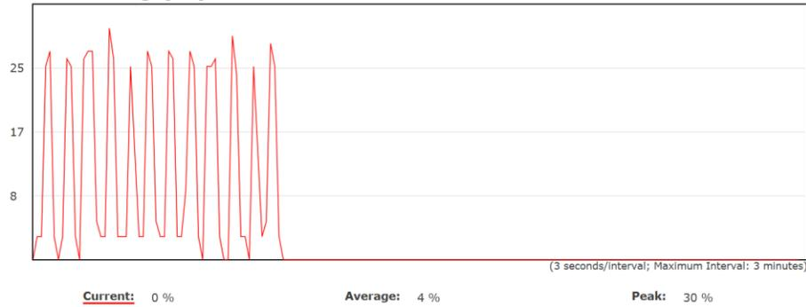
**Traffic Loading: 2.4GHz and 5GHz and Ethernet port inbound and outbound traffic by current, average and peak time.**
